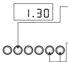
Step 4 Press & hold in the Cook Period button, the display will read 0.00 and the 'cookpot' symbol will light up. With the Cook Period button still held in set the required Cook Period using the "+" and "-" buttons. Example: 1hr 30 minutes (as shown).
