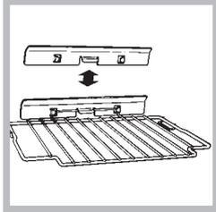
The shelf in the top oven has a heat shield fitted at the rear. The shield can be removed for cleaning and grilling, but should be replaced when using the oven for best cooking results. It has a safety stop to prevent it from being pulled out too far when attending to food.
