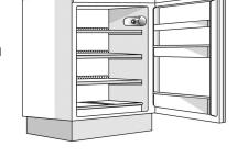
Note: Do not use sharp or pointed metal instruments to scrape off ice; do not heat the low temperature compartment artificially.
