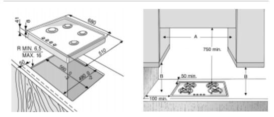
Note: If the distance "A" between the wall cabinets is between 600 mm and 680 mm, the height "B" must be a minimum of 520 mm.
