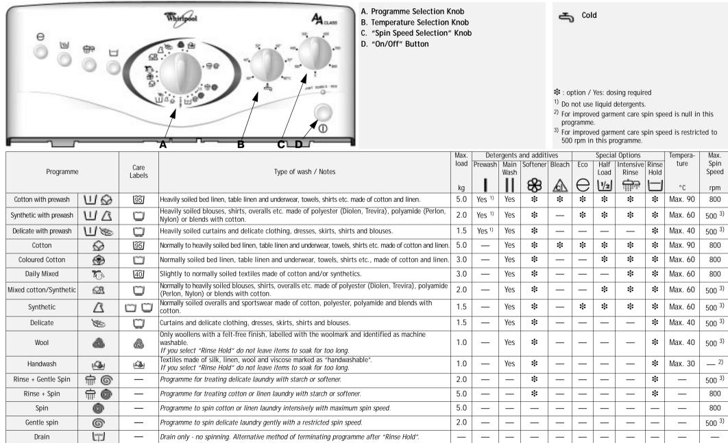
N.B. This machine is controlled by sensors. Please avoid excessive detergent dosing.
