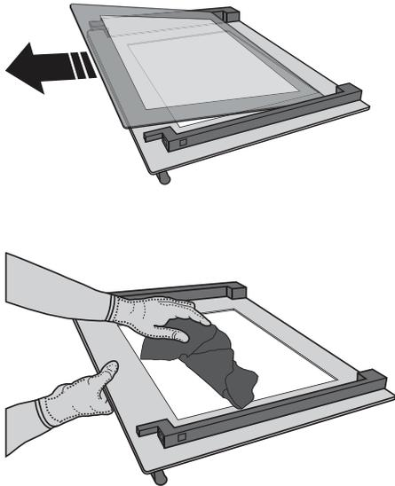
**3.** Refit the intermediate pane (marked with "R1") before refitting the inside pane: To position the panes of glass correctly, make sure that the "R" mark can be seen in the left-hand corner. First insert the long side of the glass indicated by "R" into the support seats, then lower it into position. Repeat this procedure for both panes of glass.
