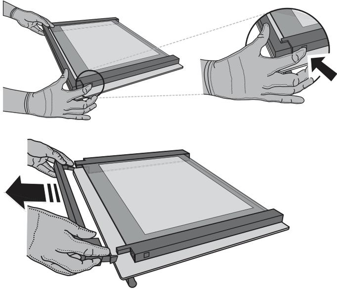
**2.** Lift and firmly hold the inner glass with both hands, remove it and place it on a soft surface before cleaning it.
