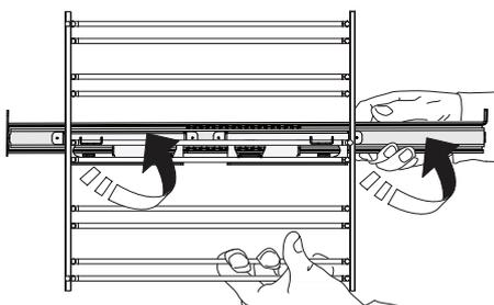
3. To reinstall the sliding guides, anchor the guide's upper clip to the shelf guide, then lower the other clip into position.
