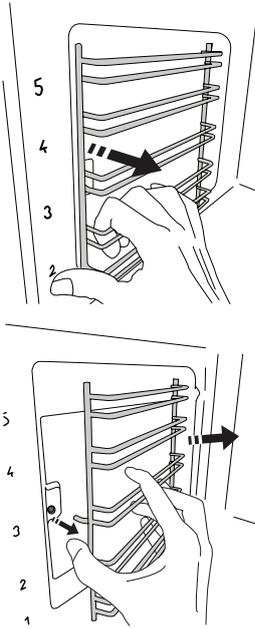
• **To reposition the shelf guides**, position them near the cavity and initially insert the two pins into their lodgings. Next, position the external part near its lodging, insert the support, and firmly press towards the wall of the cavity to make sure the shelf guide is properly secured.
