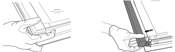
**2.** Lift and firmly hold the inner glass with both hands, remove it and place it on a soft surface before cleaning it.
