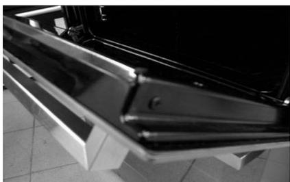
Remove screws from both side of door
