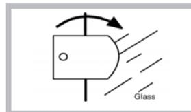
1. Turn the two securing brackets back to their original position to retain the glass and tighten the screws. (Fig. 2.)
