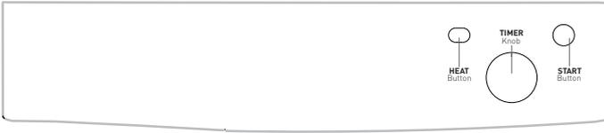
The **TIMER** knob: the **0** position switches off the dryer.
