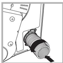
Vent Tube fitted here
