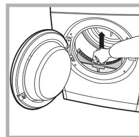
Failure to clean the filter after EVERY drying cycle will affect the drying performance of your machine. It will take longer to dry and as a result will use more electricity during drying.
