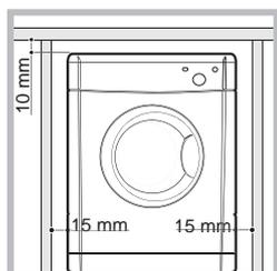
If you are going to install the appliance under a work counter be sure to leave a 10 mm space between the top and any other objects on or above the machine and a 15 mm space between the sides and any kitchen units
