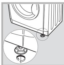
The dryer must be installed level for correct operation. When you have installed your dryer in its final location check that it is first level side to side and then back to front.
